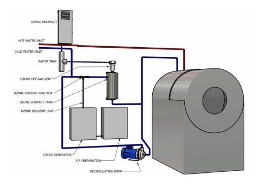
**Figure 6.** Schematic diagram of Pressurized Ozone Charge System.
