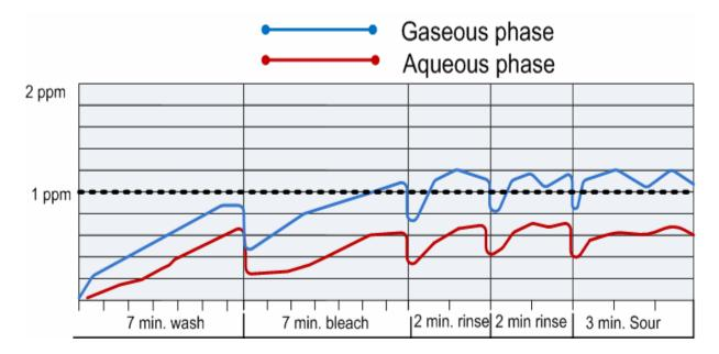
**Figure 9.** Ozone in aqueous and gaseous phases in an Ozone Diffusion washer. Ozone in gas phase controlled by means of an Aquawing ozone monitor/controller (graphic courtesy of Dave Spofford, AWOIS LLC, Auburn, NH, USA).
